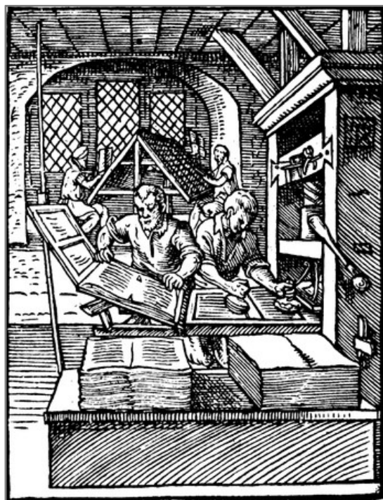
Early wooden printing press, depicted in 1568, by Jost Amman (1568). Such presses could produce up to 240 impressions per hour.
